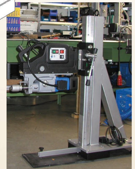
Machine rendering above shows reverse-mount motor for drilling upside down.
